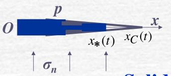
Fracture inlet x = 0**Liquid front**  $x_*(t)$  **Crack tip**  $x_C(t)$ Lag  $x_C - x_*$
