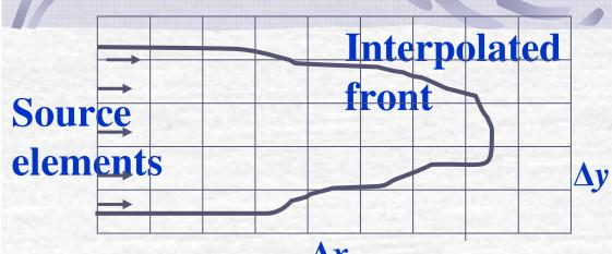
Planar fracture geometry based on rectangular boundary elements
