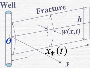
Continuity equation (no leak-off)  $\frac{\partial q}{\partial x} + \frac{\partial w}{\partial t} = 0$ Poiseuille equation (Newtonian liquid)  $q = -k_l w \frac{\partial p}{\partial x}$
